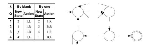
**Figure 1.** A 5-tuple TM and its transition table. The blank symbol is represented by a **0**. This machine is the 4-state Busy Beaver (Brady, 1975).
