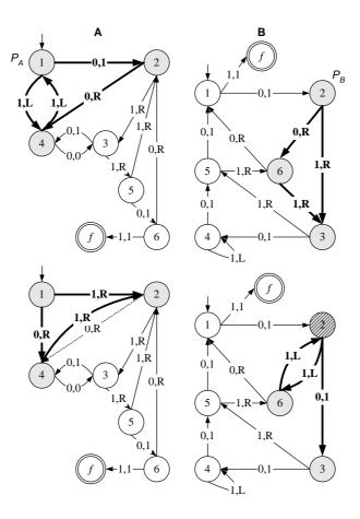
**Figure 10.** Example of Crossover. Nodes belonging to the sub-graphs are depicted in gray and transitions in bold. A dashed line represents internal transitions that weren't replaced.
